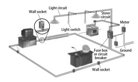
In a house, many appliances use current from the same circuit. If more appliances are plugged in on a circuit, more current will flow through the wires. As more current flows through the wires, more heat is produced in the wires. If the wires get too hot, the insulation can melt. The bare wires can touch, get hot, and cause a fire. To keep the wires from getting too hot, household circuits include either a fuse or a circuit breaker.
