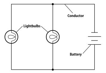
Houses, cars, and most electric systems use parallel circuits. When one path is opened, the current still flows through the other paths. One part can be turned off without turning off the whole circuit.
